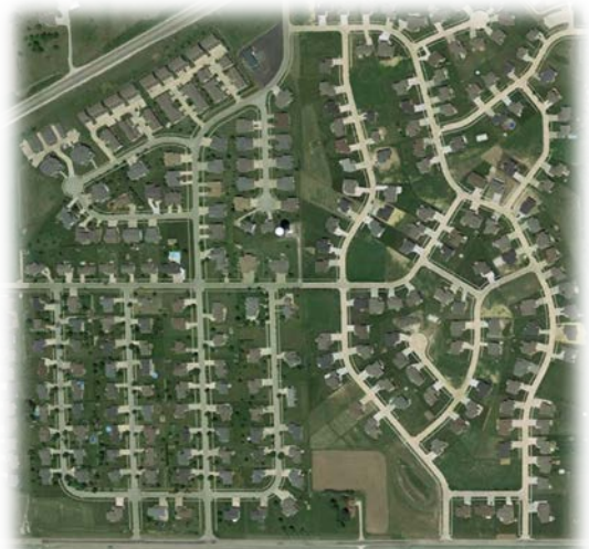
Contrast between modified grid (left) and curvilinear street patterns (right)
