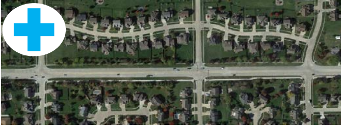
Contrast between consolidated 4-way intersections (left), and staggered 3-way intersections (right), along an arterial
