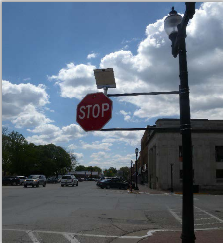
Solar powered flashing LED stop sign, mounted on light pole. This replaced a traditional stop light at Monroe and Jefferson Streets.
